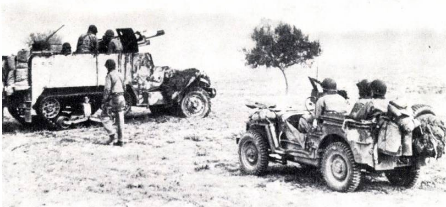
In action against German-Italian positions in Tunisia after U.S. forces invaded North Africa in 1942 is a T-19 half track (left) serving as carriage for a 105mm howitzer.
